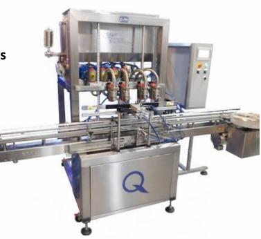
A Piston Filler utilizes a volumetric fill principle by pulling product into the cylinder from a bulk supply during the retraction of the piston. Once the cylinder is full, product is pushed out through the fill heads into waiting containers as the piston returns to the cylinder. Ideal for high viscosity products and products with particulates, piston fillers handle gels, heavy sauces, salsa, salad dressings, pastes and much more!
